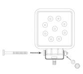
C. Attach lamp to a base. Add nut and washer to short bolt.
