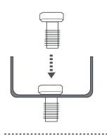
B. Assemble the "U" bracket to the bottom of the lamp, insert the long bolt through the hole and the "U" bracket.
